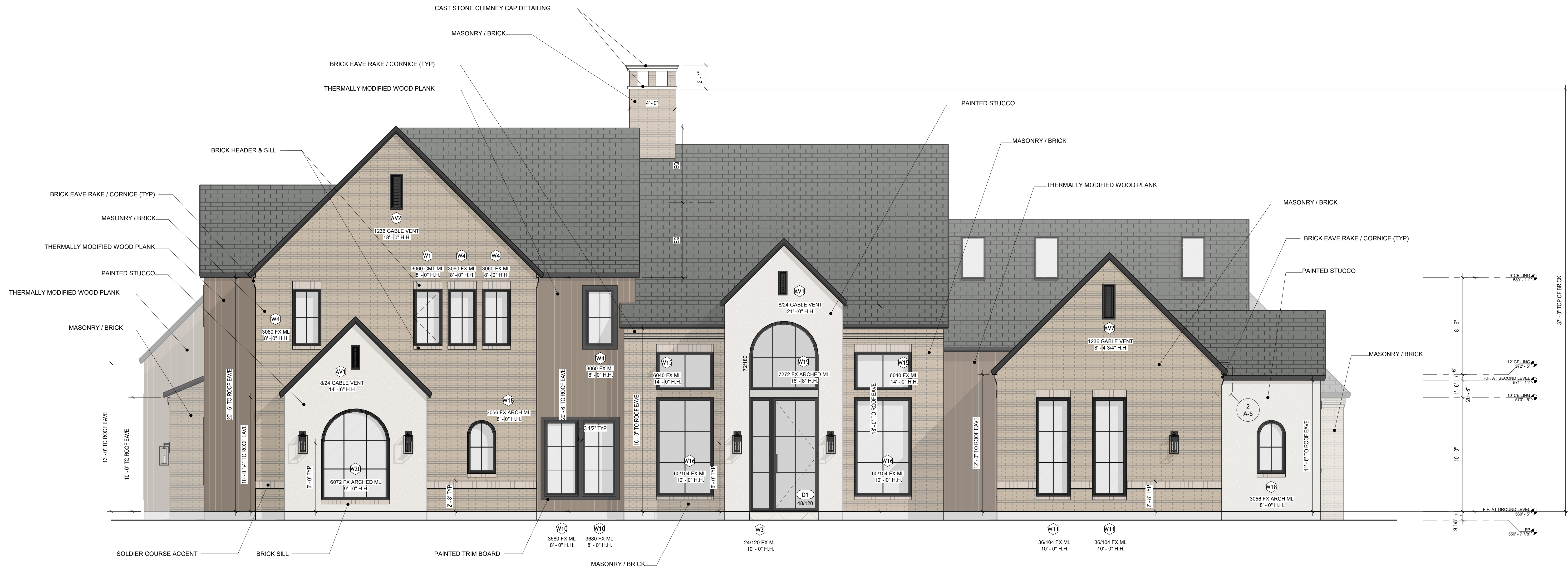
1 OVERALL ELEVATION AT FRONT FACADE 1/4" = 1'-0"
